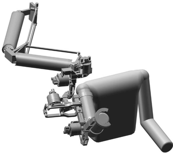
Fig. 8. Limpact exoskeleton [31], [32] uses rotation hydroelastic actuators on its shoulder and elbow joints. With the lessons learned from the Dampace, it uses the DP linkage mechanism and the external rotation center mechanisms at the shoulder axial rotation axis. The cabled design of the elbow joint of the Dampace has been replaced by a push-pull mechanism, which is stronger and requires less maintenance.
