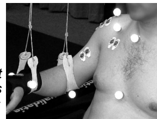
Figure 2: elbow and wrist supports, EMG pads and Vicon markers
