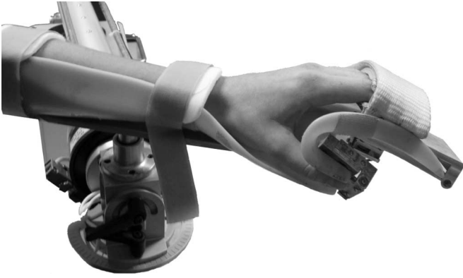
Fig. 2. Photograph of the WFFS attached to the ACT 3-D . The rigid strap shown on the fingers is secured to the finger plate to restrain the fingers and does not make contact with the orthosis. A similar strap restrains the thumb (not shown).
